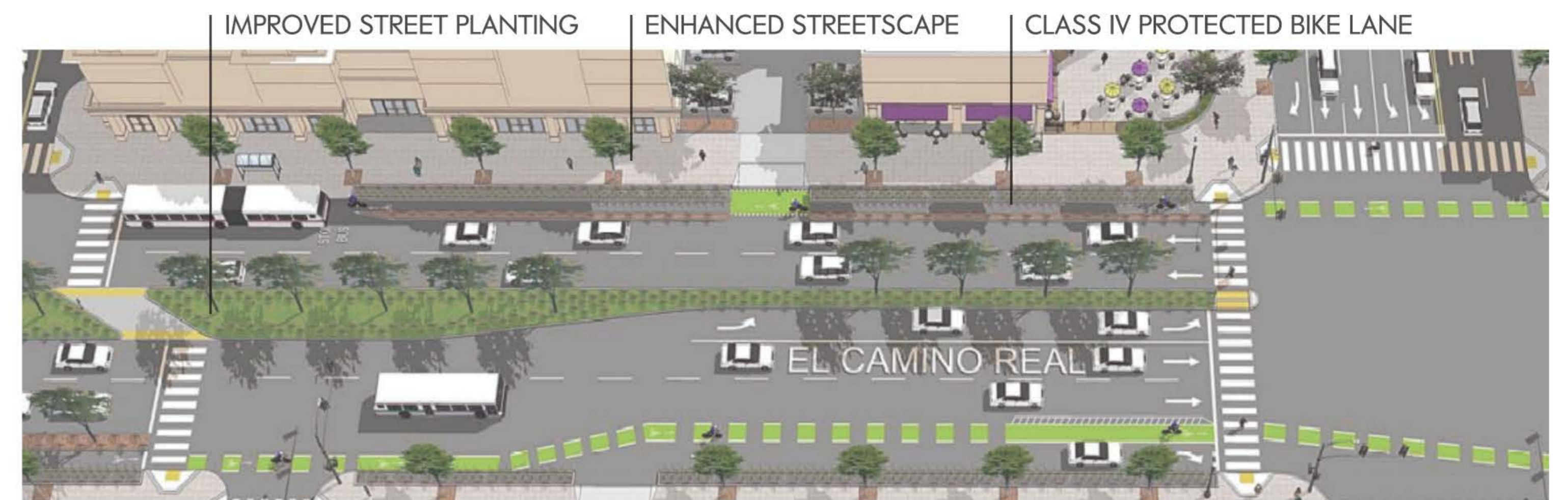
CORRIDOR PLAN RECOMMENDED IMPROVEMENTS AT JEFFERSON AVENUE INTERSECTION
